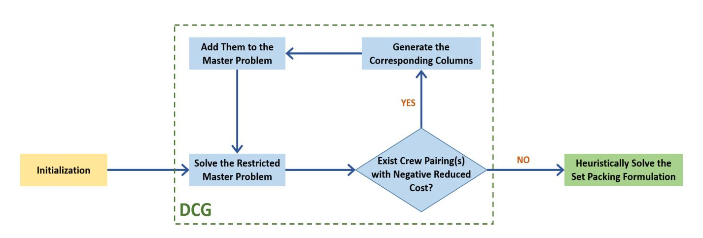
The pricing problem of the DCG is modeled as a shortest path problem with resource constraints (SPPRC) on a flight-based network.
